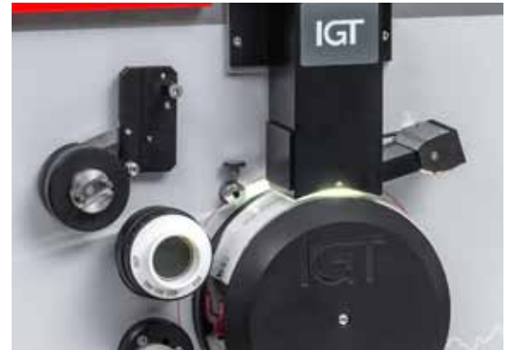
IGT Pick ISO 3783: the camera is scanning
